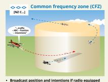
Anticollision and/or landing lights should be on if so equipped
