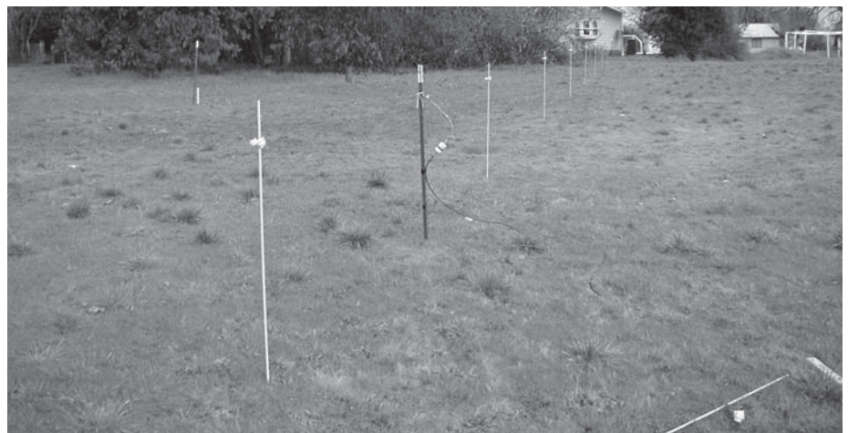
Figure 8 — Test antenna supported with F/G wands. [Rudy Severns, N6LF, photo.]
