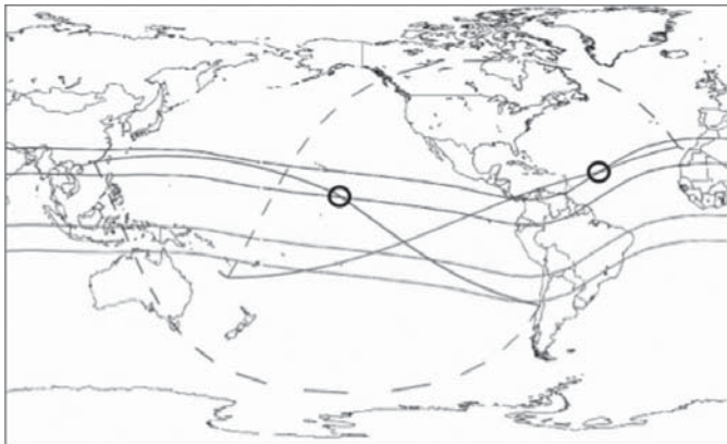
Figure 14 — Both skew paths start as south-lane TEP and then are redirected upon entering a later lane (circles). The path from CE then does a 2F2 hop in the north lane to BA. The FK8 path crosses the north lane and runs into it again, and is redirected to EA8. [G.Projector map and overlays.]
