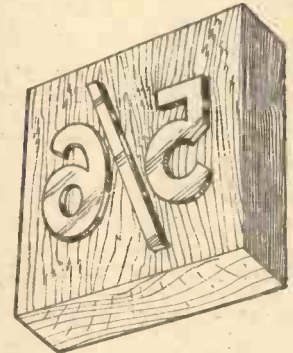
Fig. 5.—Larger stamps, as shown, can be cut from sheet rubber and glued to a wooden base.
