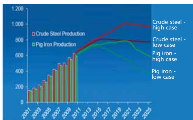
Fig 5 Pig iron and crude steel production in China, 2001-2025 (Mt) Source: R McLaughlin Hatch Associates
