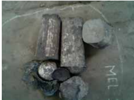
Fig 1 Cast ingots of HCFeMn fines cast from a 28kg steel scrap starting pool with 21kg HCFeMn added at 3kg every 3 minutes
