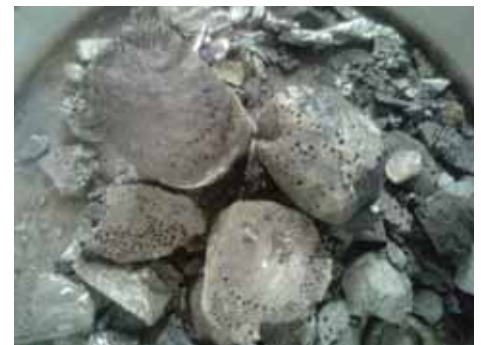
Fig 4 Pieces of cast ingot broken during stripping when 33kg of SiMn fines were added to a 11kg scrap steel starting pool
