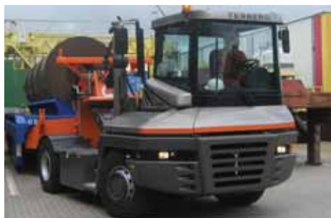
Fig 2 The driver's cabin is ergonomically designed and its suspension protects the driver on the rough roads around the works
