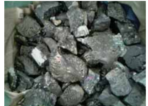
Fig 2 Broken SiMn lumps cast from 15kg steel scrap starting pool with 30kg SiMn fines added at 3.0kg every 5 minutes
