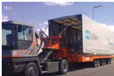
Fig 3 Covers have been designed to protect the coils from bad weather
