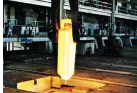
Fig 3 Solidified ingots being charged to a soaking pit while still hot from casting
