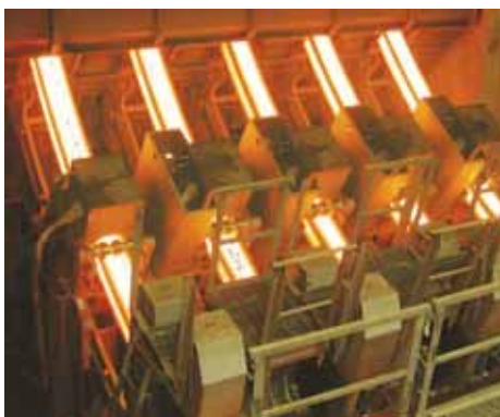
Fig 5 Multistrand bloom caster simultaneously casting five strands
