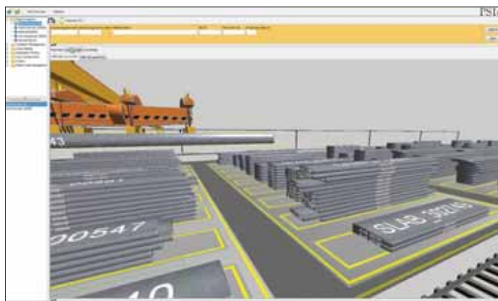
Fig 3 Slab yard overview in PSImetals Logistics providing different levels of detail (yard field, detailed spaces, position in pile) Source: PSI Metals
