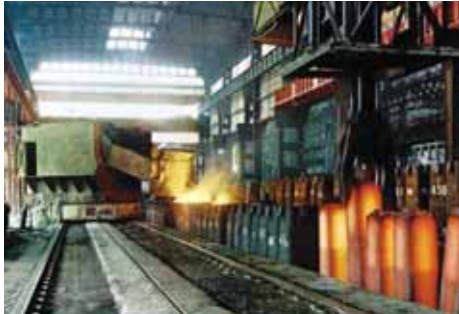
Fig 2 Solidified steel ingots in foreground and teeming into mould in background
