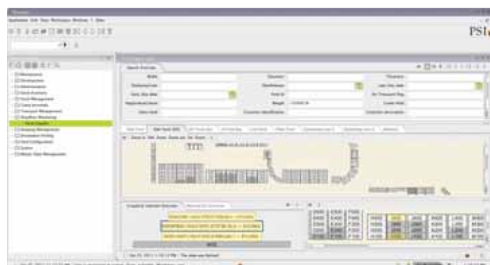
Fig 3 Slab yard overview in PSImetals Logistics providing different levels of detail (yard field, detailed spaces, position in pile) Source: PSI Metals
