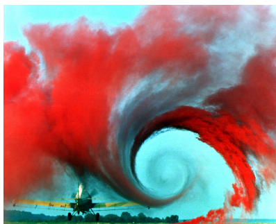
(a) Landing agricultural airplane's wake (b) Visualization of FEM-based computer vortex, visualized by colored smoke rising simulation of turbulent flow, showing velocity streamlines.
