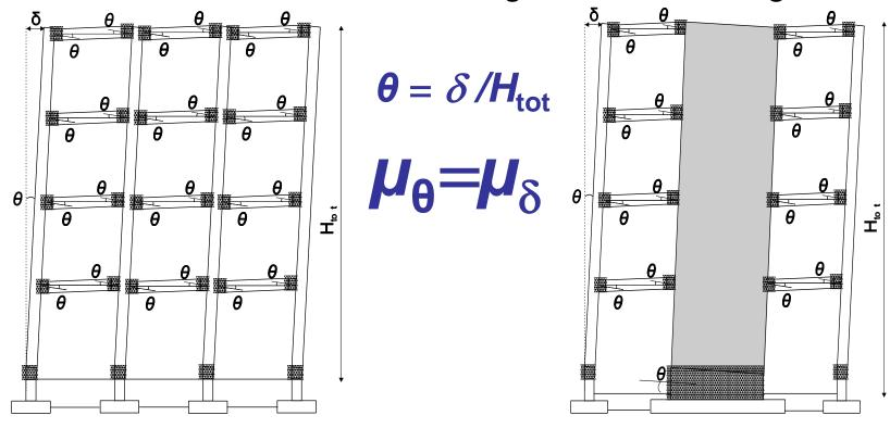
Strong-column/weak-beam capacity design: ∑M<sub>Rc</sub>≥1.3∑M<sub>Rb</sub>
