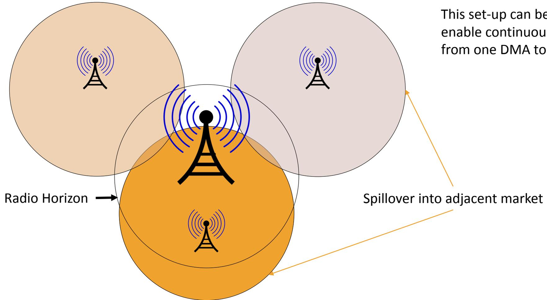
This set-up can be used to enable continuous service from one DMA to another
