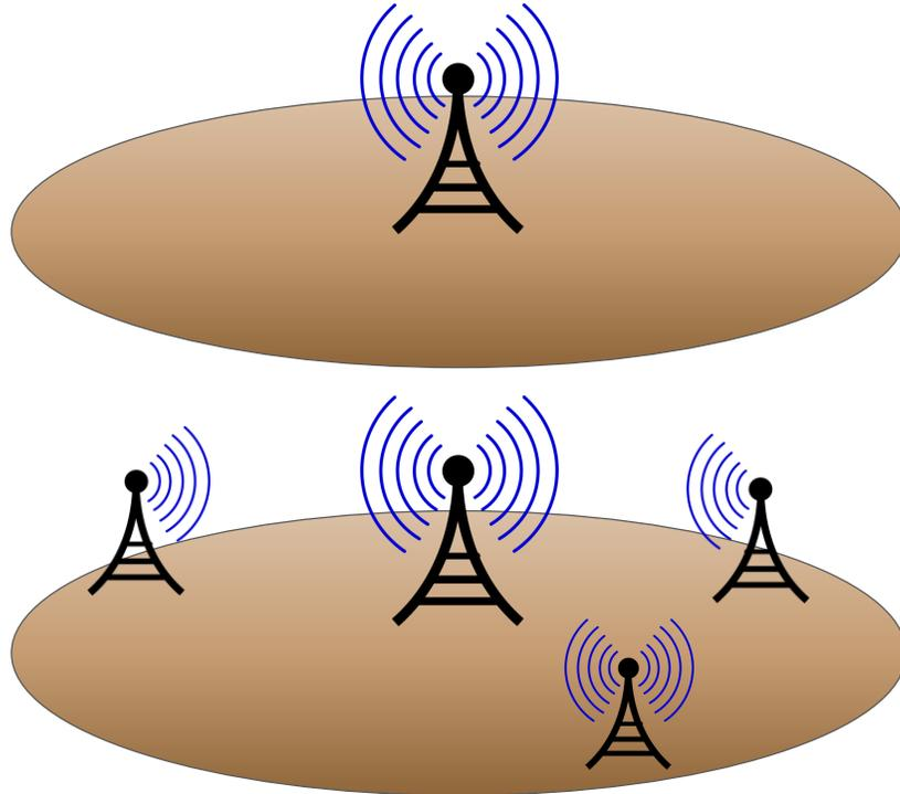
SFN with multiple transmitters increases coverage by boosting SNR in coverage holes
