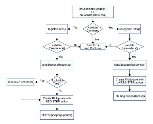
Figure 15: Verb dispatch workflow of the RIB Manager
