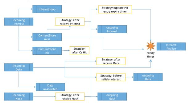
Figure 7: Pipelines and strategy: overall workflow
