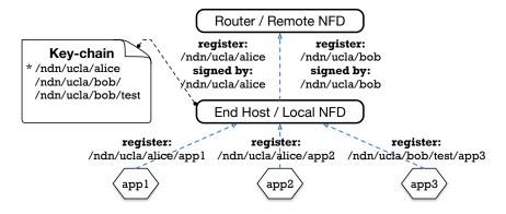
Figure 18: An example of prefix propagation
