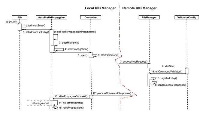
Figure 19: The simplified workflow of a successful propagation
