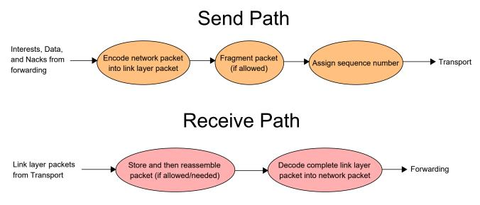
Figure 3: GenericLinkService Internal Structure
