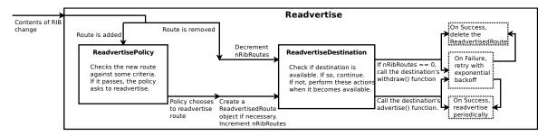
Figure 16: The simplified structure an operation of the Readvertise module.
