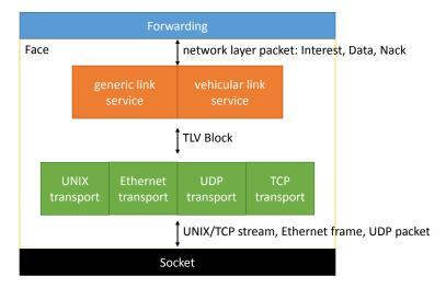
Figure 2: Face = LinkService + Transport
