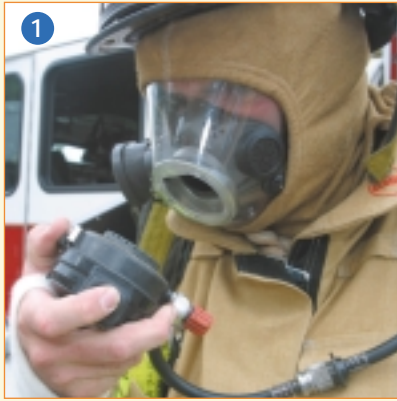
1 Remove your gloves. Remove the regulator from the face piece or disconnect the low-pressure hose from the regulator.
