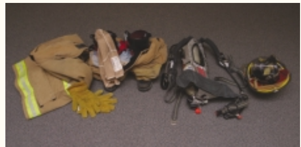
Figure 2-12 The complete structural firefighting ensemble consists of a helmet, coat, trousers, protective hood, gloves, boots, SCBA, and PASS device.
