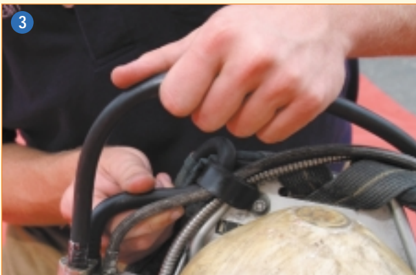
3 Check condition of all hoses while pressurized.
