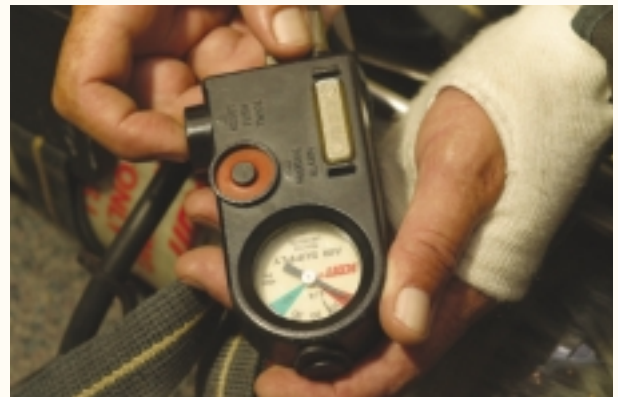
Figure 2-20 A PASS can save a fire fighter's life.
