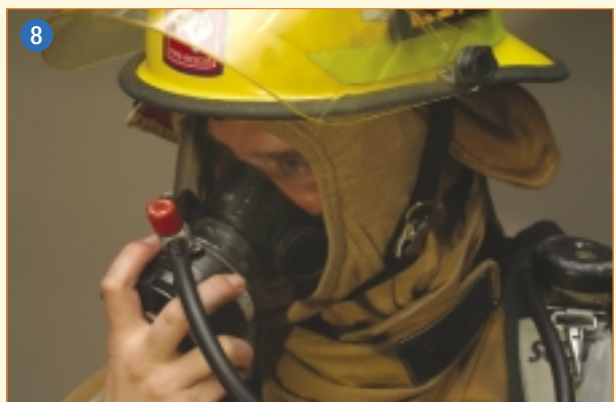
8 Install the regulator on your face piece or attach the low-pressure air supply hose to the regulator.
