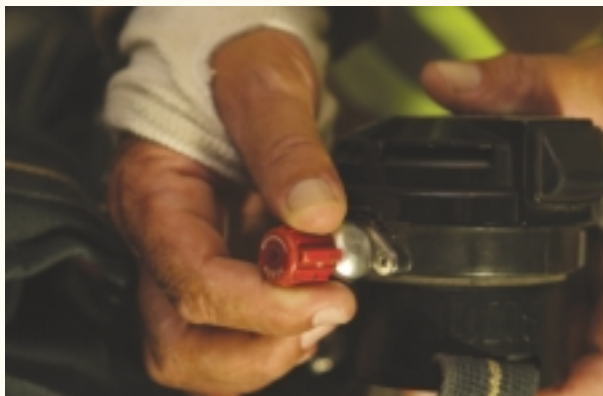
Figure 2-29 The SCBA emergency by-pass valve is used if the regulator malfunctions.
