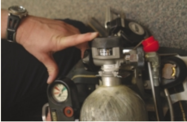
Figure 2-30 A PASS device can be integrated into an SCBA.
