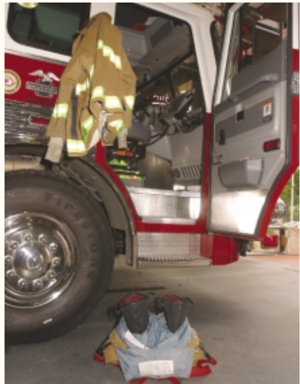
Figure 2-5 Protective clothing should be properly positioned so you can quickly don it.
