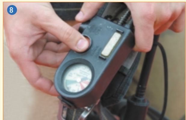
Check function and activation pressure of low-air alarm. Close by-pass valve and restore unit to ready condition.
