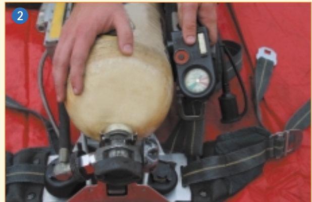
2 Check air-cylinder pressure. Turn on the air-cylinder valve and check gauge pressure.
