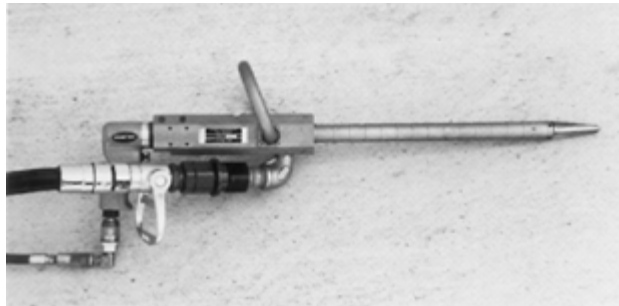
FIGURE 11.4.4 Skin Penetrator Agent Applicator Tool (SPAAT).
