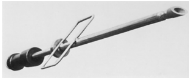
FIGURE 11.4.3 Aircraft Skin Penetrator Nozzle.
