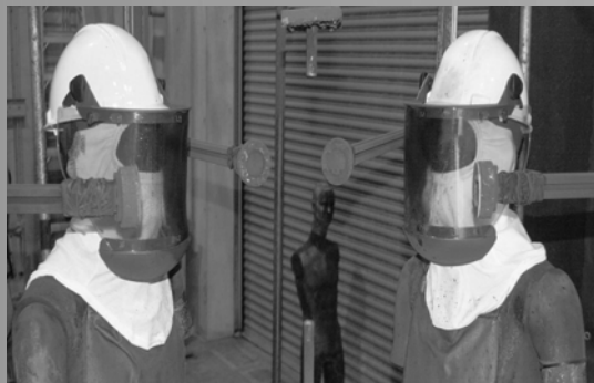
Arc Rating (ATPV) = 10.9 cal/cm 2
