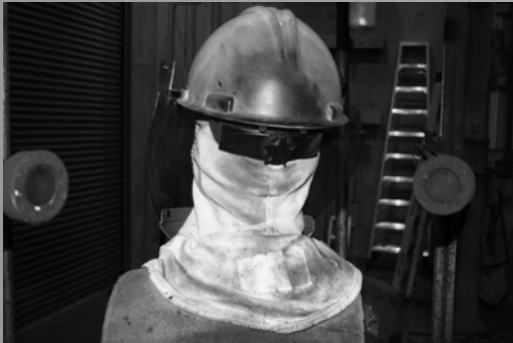
Arc Rating (ATPV) = 30 cal/cm 2
