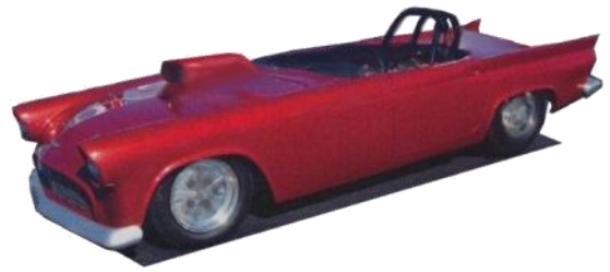
Radiused and recessed flanged drivers compartment for flush mounting of removable "contoured" tonneau cover and drivers windshield fairing
