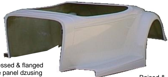
Raised & radiused rear fenders with edge bead
