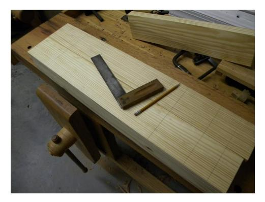
I then moved on to the legs assemblies. The legs are simply three pieces of  $1 \frac{1}{2}$  in x  $4 \frac{1}{4}$  in stock glued up, planed and jointed to 4 in x 4in. I then laid out 1 in x  $3 \frac{1}{4}$  in mortises for an upper and lower stretcher that connects the legs.
