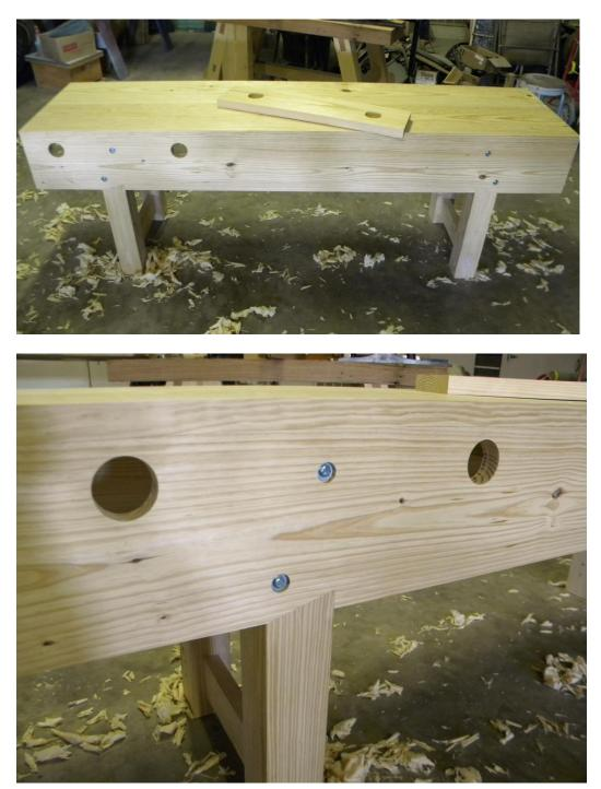
Last thing was to bore the 2 5/8 in holes for the vise screws and I made vise chop from a piece of  $1\frac{1}{2} \times 31$  in stock. The wooden vise screws are from Lake Erie Toolworks; they were perfect as always.
