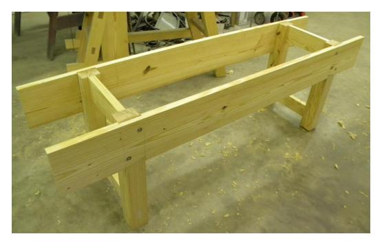
I then glued the skirts to the underside of the top and clamped it all up. By bolting the leg assemblies in beforehand they will hold the skirts square to the top and keeps the spacing for the leg assemblies is perfect.
