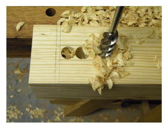
These are pretty straight forward mortise and tenon joints. The upper stretcher's tenons are set down from the top of the legs about  $1\frac{1}{2}$  in. The lower stretcher is placed about 3 in from the bottom of the leg. I used a 7/8 in auger and bored out the majority of the waste and the squared up the mortise walls with a chisel.
