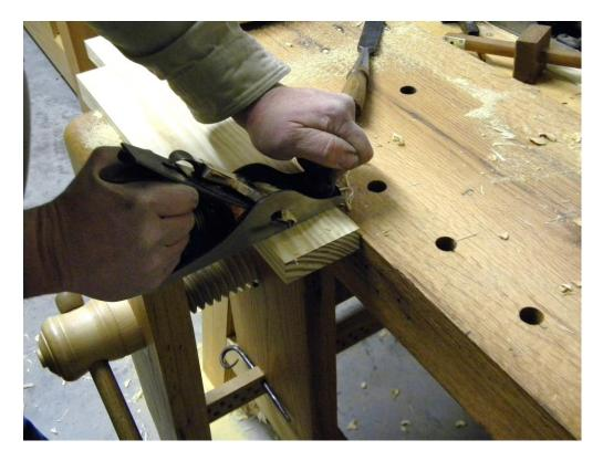
Using a mortise gauge I scribed the 1 in. tenons on the end and a cutting gauge to lay out the shoulders. I then sawed the cheeks and shoulders, once that was complete I cleaned them up with a chisel and a plane.
