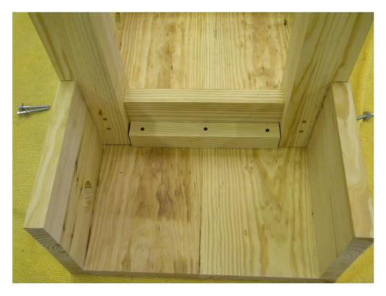
I also added two  $2 \ge 2$  in stiffeners at the top of each leg assemblies. These also capture the top stretcher of the leg assemblies to help support them as well.
