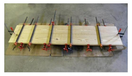
I started with the top first on this bench. The whole bench is made from lumber yard yellow pine 2 in x 12 in x 16 ft framing lumber. After letting the lumber acclimate in the shop for a few weeks, I picked out the two flattest and straightest 8 ft pieces for the top. I jointed the edges and glued them together. Once the top was glued I could determine the maximum width I could get out of the two boards, in this case was about 21  $\frac{1}{2}$  in.
