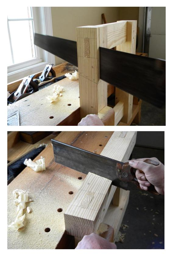
I then used a marking gauge to lay out a line on the legs the depth of the shoulder needed to be; in this case about 1 in deep. I used a rip saw and cut to this line down to the angle.
