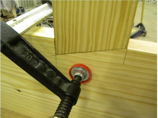
When the legs were all fitted to the dados in the skirts I bored holes for two 3 in. lag bolts
