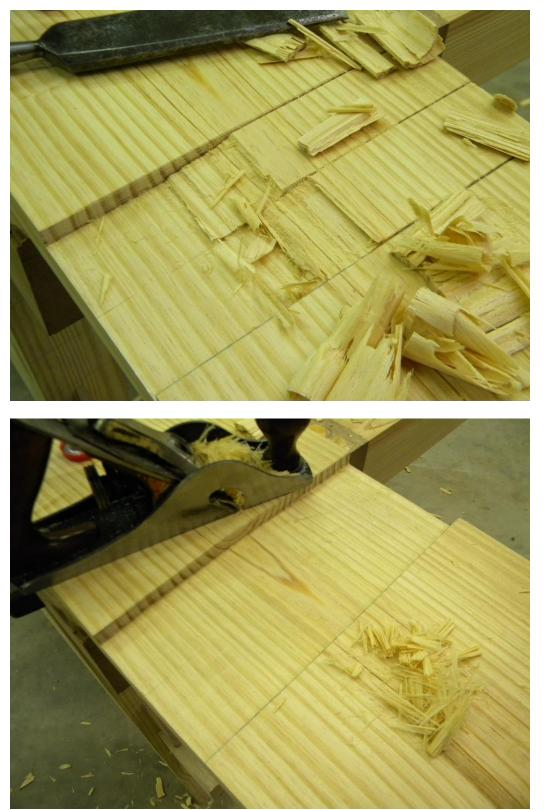
I then cut two ½ in deep by 4 in. wide dados about 11 ½ in. in from the ends of the skirts. The leg assembles will slide into these and be secured by bolts a little later. These are simple to make, I cut the shoulders with a back saw to the exact width of the legs and
