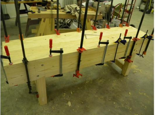
With the top and skirts assembled I then added four stiffeners evenly spaced under the top. These are  $1\frac{1}{2}$  in x 3 in pieces of wood attached with screws only; no glue. I enlarged the screw holes in the stiffeners a bit to allow for seasonal expansion and contraction.
