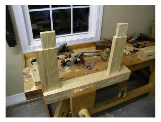
With the joints fitted I bored two 3/8 in peg holes in each mortise then bored the tenons with the peg hole moved toward the shoulder slightly to drawbore the joint. I glued and clamped the joints then drove in the pegs.
