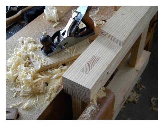
I used a plane to finish up the shoulder, stopping when the front of the leg and skirt were flush.
