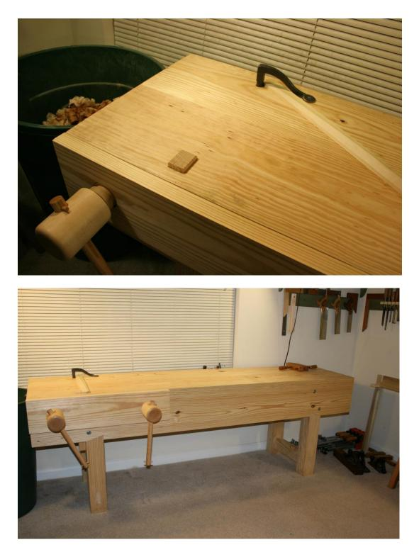
The finished dimensions of this bench are 90 in long x  $21 \frac{1}{2}$  wide x 30 in tall. Overall weight is 200 lb.
