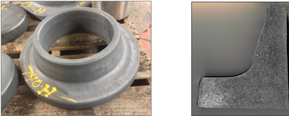
Figure 7. a) Appearance of weld-neck flange forging; b) Etched cross-section
