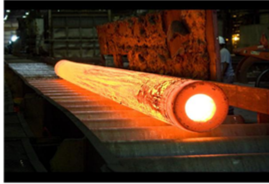
Figure 6. Heavy wall 740H pipe extruded at Wyman-Gordon, Houston TX.
