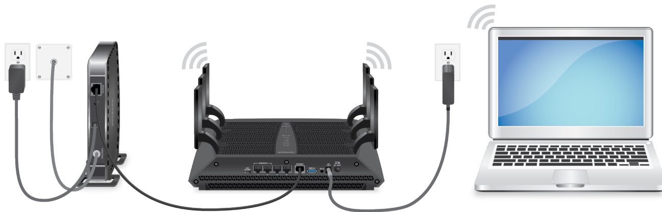
Figure 5. Cable your Router
