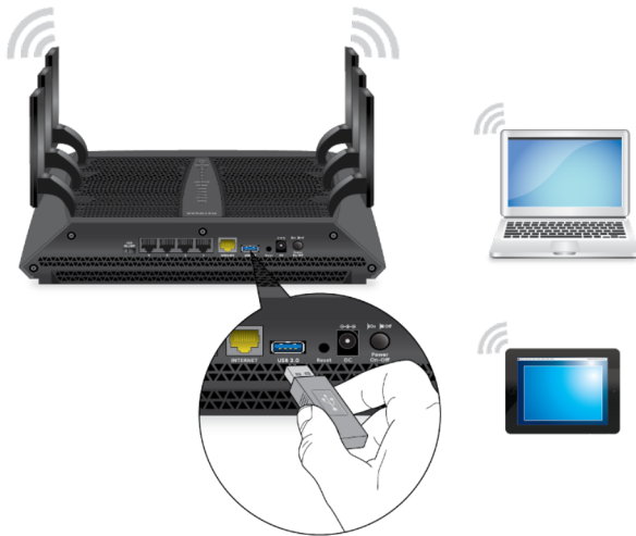
Figure 7. One USB 3.0 port is located on the back panel of the router
