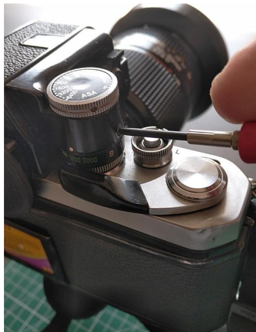
Reposition the screw for closing off the set screw access hole.
