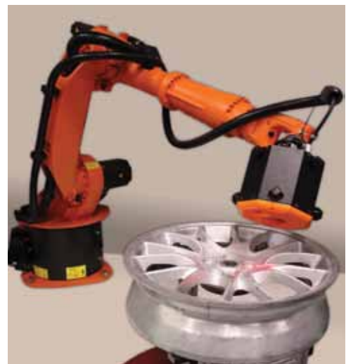
Fast repetitive laser scanning for in-production-line inspection
