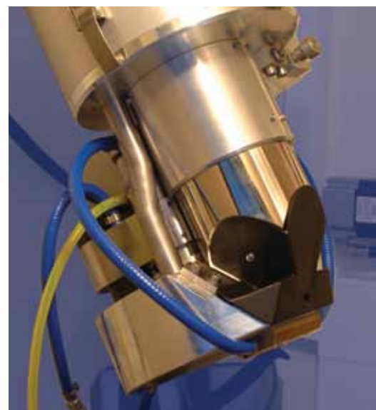
An X-ray source with rotating target boosts X-ray flux by up to 5 times, enabling customers to obtain faster CT data acquisition or achieve higher CT data accuracy in the same time span.
