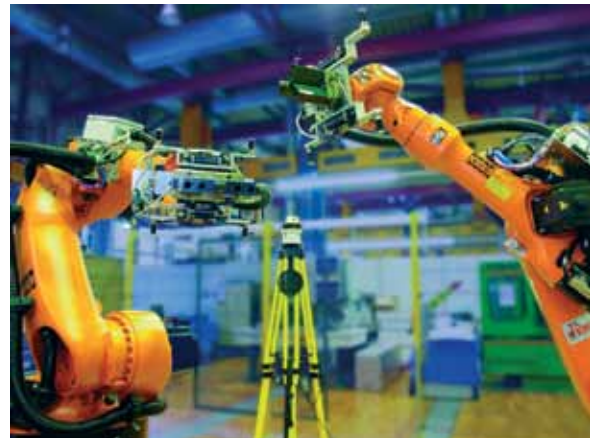
Adaptive Robot Control - driven by Optical CMM or iGPS - establishes a closed feedback loop that nearly eliminates the influence of robot warm-up, drift and backlash
