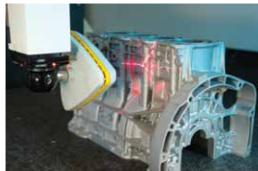
The scanner's high field of view depth results in major time savings when inspecting automotive cast parts.
