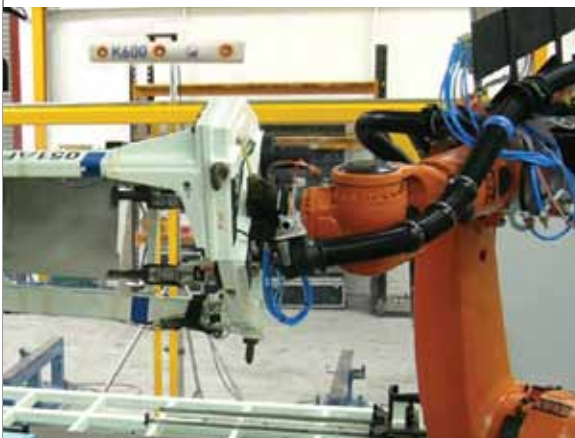
Adaptive Robot Control - driven by Optical CMM or iGPS - establishes a closed feedback loop that nearly eliminates the influence of robot warm-up, drift and backlash
