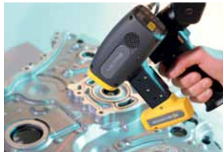
MMDx scanner is available in 50/100/200mm stripe width and MMCx features a 80/160mm stripe width
