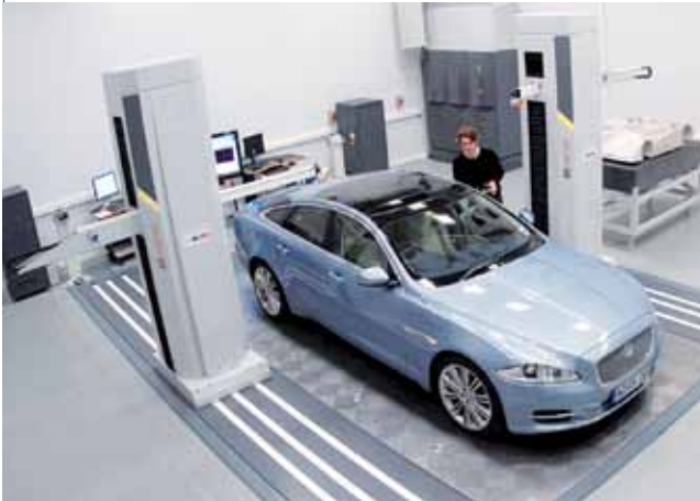
LK H-R premium series twin-rail mounted horizontal arm CMM with walk-on covers
