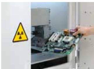
Large door with automatic interlocked X-ray off function
