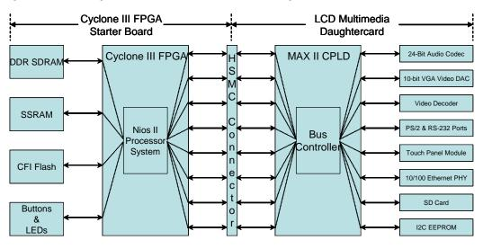
Figure 3–1. Block Diagram of Nios II Embedded Evaluation Kit, Cyclone III Edition
