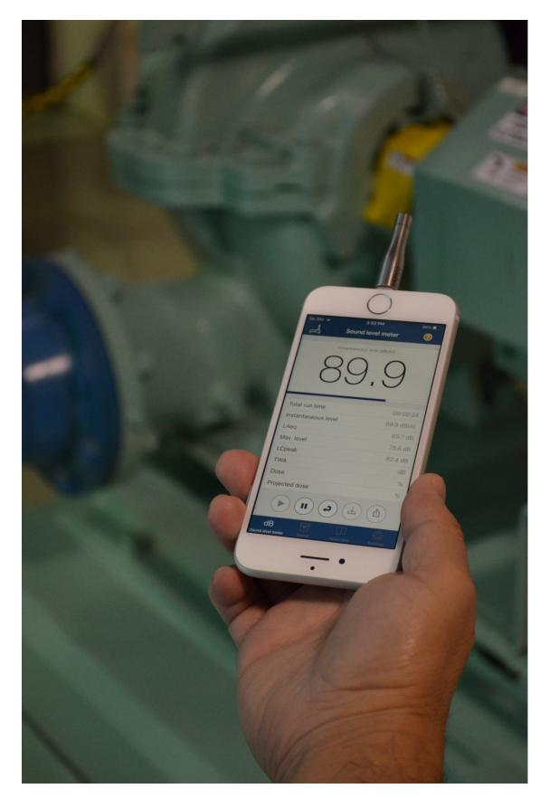
Figure 1. The main screen of the NIOSH SLM app (shown with an external microphone on iPhone 8)
