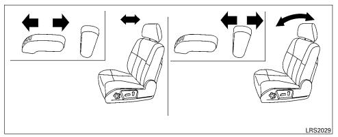
The reclining feature allows adjustment of the seatback for occupants of different sizes for added comfort and to help obtain proper seat belt fit. See "Precautions on seat belt usage" later in this section. Also, the seatback can be reclined to allow occupants to rest when the vehicle is stopped and the shift selector is in P (Park).
