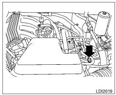
**VQ40DE engine**CHECKING ENGINE OIL LEVEL
