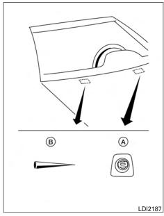
Be careful not to let anything get into the washer nozzle (a). This may cause clogging or improper windshield washer operation. If something gets into the nozzle, remove it with a needle or small pin (B).
