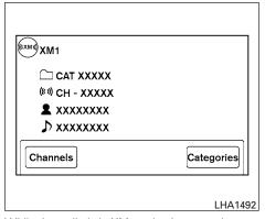
While the radio is in XM mode, the operation can be controlled through the touchscreen. Touch the "Channels" key to display a list of channels. Touch a channel displayed on the list to change to that channel. Touch the "Categories" key to display a list of categories. Touch a category displayed on the list to display options within that category.
