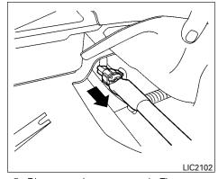
5. Disconnect the power supply. The connector may need to be accessed from the driver's door side of the seat by reaching underneath the seat.
