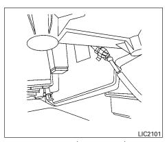
The harness cap (if so equipped) is taped to the harness underneath the inside of the center console. Remove the tape to remove the cap.
