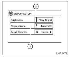
Other items are adjusted by selecting one of a set number of conditions. For example, the Display Mode can be set to "Automatic", "Day" or "Night". To adjust this type of item, touch the item ①. The item will cycle through the available settings and the red indicator lights to the left of the setting condition ② will come on or turn off accordingly.
