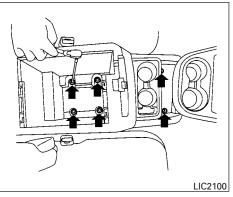
4. Remove 4 bolts located inside the console and 2 in the front storage tray.
