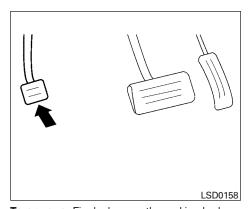
**To engage:** Firmly depress the parking brake.
