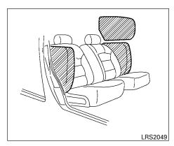
Front seat-mounted side-impact supplemental air bag (if so equipped) and roof-mounted curtain side-impact supplemental air bag (if so equipped) systems
