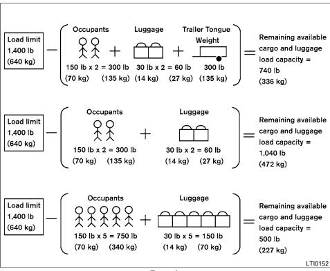
Steps for determining correct load limit
