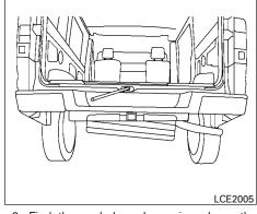
Find the oval-shaped opening above the middle of the rear step bumper. Pass the J-shaped end of the jack rod through the opening and direct it toward the spare tire winch, located directly above the spare tire.
