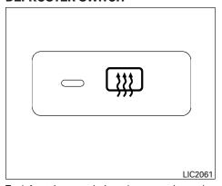
To defrost the rear window glass, start the engine and push the rear window defroster switch on. The rear window defroster indicator light comes on. Push the switch again to turn the defroster off.
