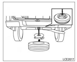
To reinstall the wheel, insert the tire chain through the wheel. Be sure the rubber spacer is centered on the wheel before lifting. Use the assembled jack rod and slowly rotate the winch clockwise to raise the wheel to the vehicle.
