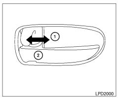
Inside lock – front driver and passenger LOCKING WITH INSIDE LOCK KNOB
