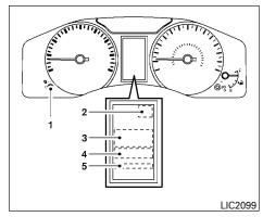
The vehicle information display is located between the speedometer and the tachometer.
