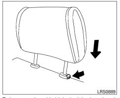
To lower, push and hold the lock knob and push the head restraint down.
