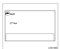
Press the AUX button to play a compatible device plugged into the AUX IN jack. The AUX button is also used to switch the audio system to a source plugged into the USB input jack in the center console. When a device is plugged into the AUX IN jack while another device is plugged into the USB input jack, the AUX button is used to toggle between the two functions.
