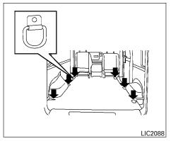
Do not apply a load of more than 1,124 lbs (5,000 N) to a single D-ring.
