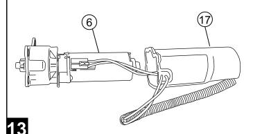
Install motor mounting bracket using the three M6x12 bolts. Then mount motor using the two M6x16 countersink bolts. Use thread locking compound.
