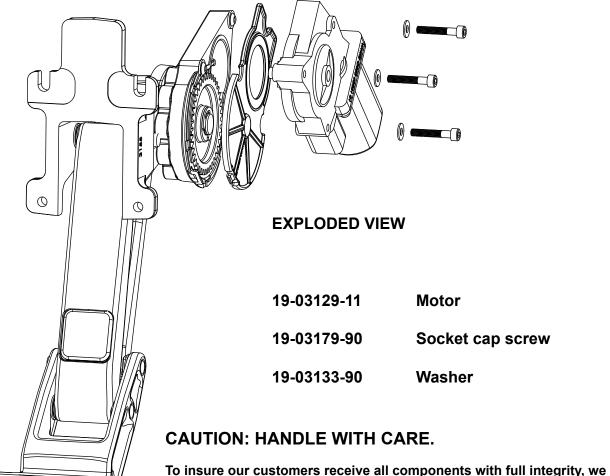
To insure our customers receive all components with full integrity, we pack the motors seperate from their linkage assemblies. This requires that the installer position and fasten the motor before continuing with the install. Please follow the instructions below and handle the assembly carefully.
