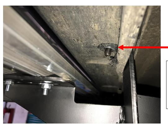
A small hole will need to be cut in the sill cover to allow the T-Bolt to come through cover (otherwise the tray will poke down.) You will need to use a T-Bolt to fit the brackets to the chassis and the sill. There are 2 locations.
