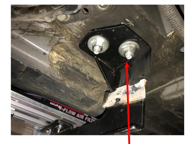
You have to insert the U-bolt through the 1<sup>st</sup> hole and drop it down through the 2<sup>nd</sup> hole.
