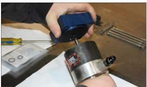
**Step 3:** Remove upper housing from pump body
