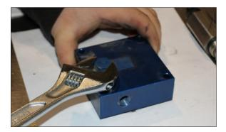
**Step 4:** Remove 11/16" bolt and block off plate from upper housing.
