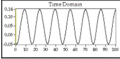
Figure 6: I(t) . V_{os} \approx 0.3 V, response period \approx 15 samples.
