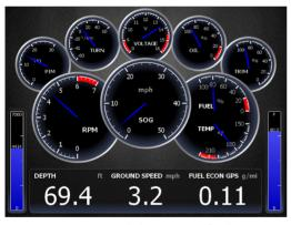
Gauge Page on HDS displaying engine interface data.
