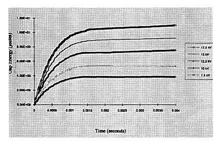
Figure 10. Gap energy vs. Voltage, High Voltage Source
