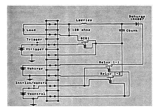
Figure 6. Mutual Inductance Particle Velocity (MIPV) Box Schematic.
