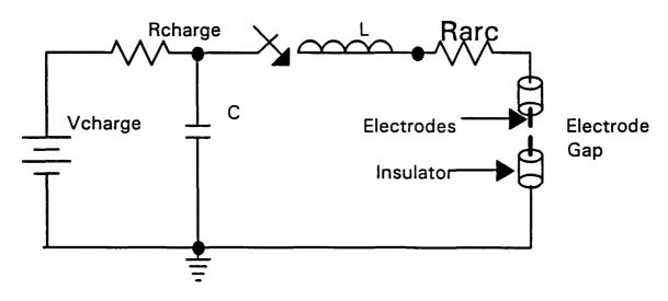
Figure 5. Typical Discharge Circuit.
