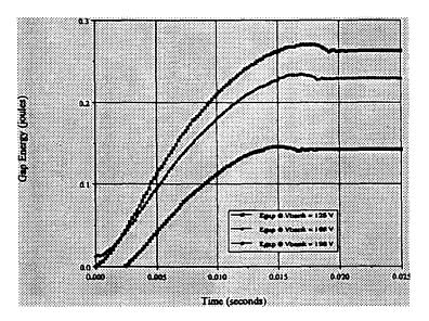
Figure 9. Gap Energy vs. Voltage, Standard NMERI DC Source
