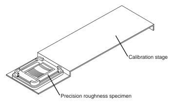
2. Mount the SJ-201P on the calibration stage.
