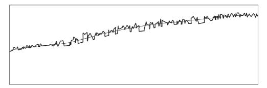
4. Original input data is compensated with reference to the second mean line.
