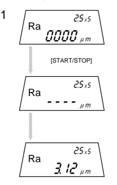
Press the [START/STOP] key in the measurement mode.
