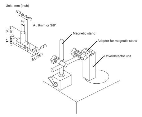
• Attaching the adapter for magnetic stand
