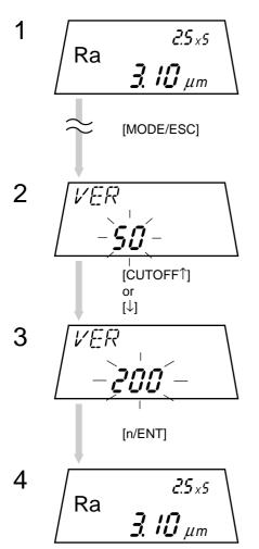
Press the [MODE/ESC] key several times in the measurement mode until "VER" (vertical magnification setting mode) is displayed.
