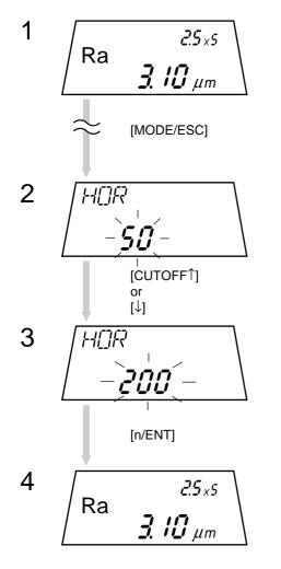
Press the [MODE/ESC] key several times in the measurement mode until "HOR" (horizontal magnification setting mode) is displayed.
