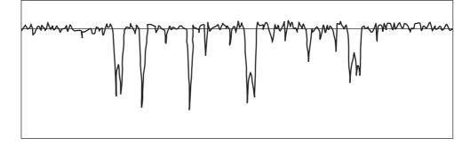
**TIP** The filters specified in DIN4777 are used for calculating both the first and second mean lines. For information about this, refer to section 10.1.3, "Evaluation according to DIN".
