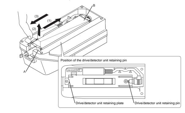
**IMPORTANT** Do not hold the detector when detaching the drive/detector unit. Otherwise, the detector may be damaged.
