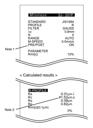
Note 1: The "Preliminary length" ON/OFF setup indicates the presence/absence of pre-travel and post-travel length setup.
