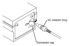
• If the AC-adapter is connected to the display unit while it is on, recharging of the battery will automatically start. The low battery voltage alarm indicator turns on during charging and goes off if the battery is fully charged.
