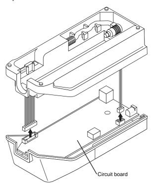
5. Remove the battery pack from the display unit.
