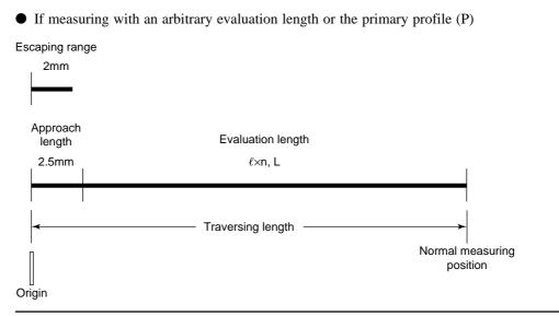
**TIP** If measuring the roughness profile without pre-travel and post-travel lengths is selected, calculation is performed with the pre-travel and post-travel data assumed to be folded (nulled).
