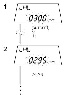
Remains in the calibration mode, ready for the entry of a numeric value. "03.00" flashes.
