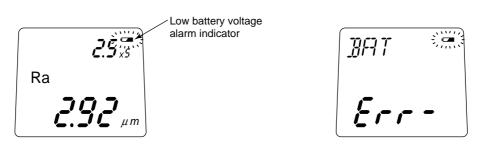
If the low battery voltage alarm indicator is flashing, recharge the built-in battery as soon as possible.
