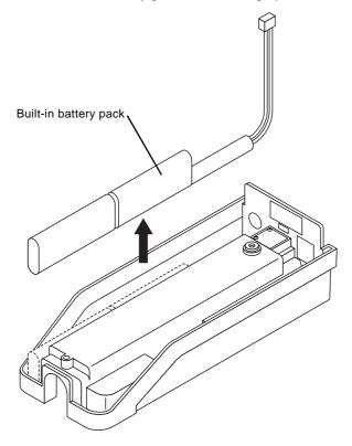
6. Place a new battery pack inside the display unit.
