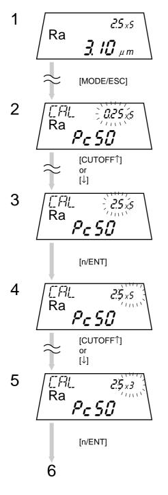
In the measurement mode press the [MODE/ESC] key until the calibration condition setup mode is entered.
