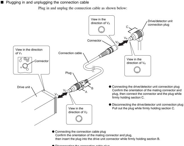
Disconnecting the connection cable plug While holding the section A, slide A towards B, then pull out the plug.
