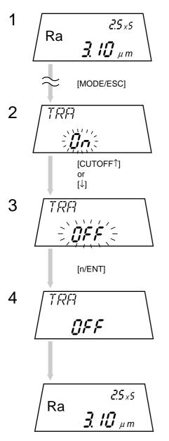
In the measurement mode press the [MODE/ESC] key until the pre-travel/post-travel length setup mode is entered.
