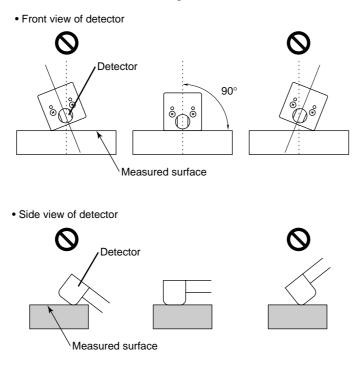
**NOTE** If calibrating the SJ-201R, check whether the detector is parallel with the measuring surface using the detector position display mode. For information about the detector position display mode, refer to "3.4.5 Displaying the detector stylus position".
