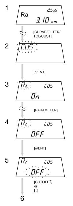
In the measurement mode press the [CURVE/FILTER/TOL/ CUST] key four times.
