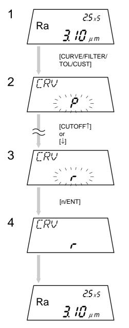
Press the [CURVE/FILTER/TOL/CUST] key several times in the measurement mode.
