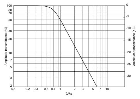
Transmission characteristic of PC50 (Gaussian)
