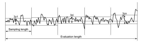
• Profile peak/highest peak and profile valley/deepest valley of assessed profiles A portion that projects upward (convex) from the mean line of the assessed profile is called the "profile peak", and that which projects downward (concave) is called the "profile valley".
