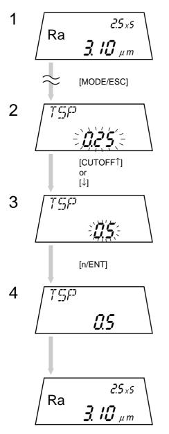
In the measurement mode press the [MODE/ESC] key until the traversing speed setup mode is entered.
