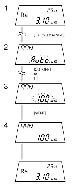
In the measurement mode press the [CAL/STD/RANGE] key three times.
