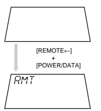
When the power is off (auto-sleep mode) press the [POWER/ DATA] key while holding down the [REMOTE←] key.
