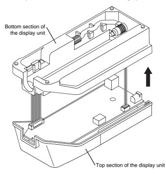
3. Gently remove the bottom section of the display unit.
