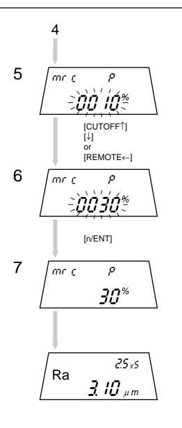
⇒ Switches to the input wait state for the slice level of parameter mrc.
