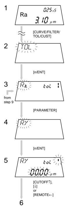
In the measurement mode press the [CURVE/FILTER/TOL/ CUST] key three times.
