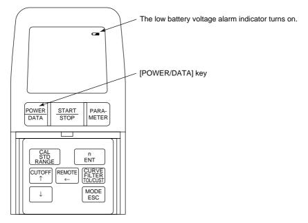
Recharging starts and the low battery voltage alarm indicator turns on.
