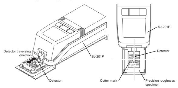
4. Confirm that the detector is parallel to the measured surface.
