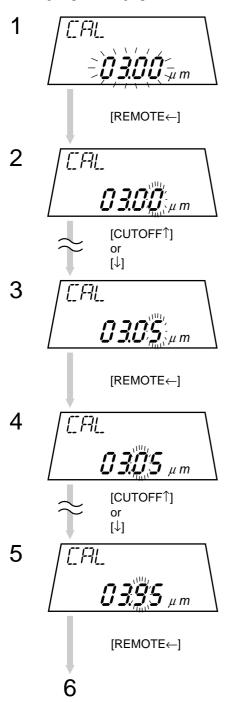
Remains in the calibration mode, ready for the entry of a numeric value. "03.00" flashes.
