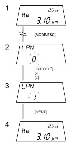
Press the [MODE/ESC] key several times in the measurement mode until "LAN" (print language setting mode) is displayed.
