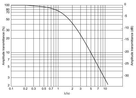
Transmission characteristic of 2RC 75 filter
