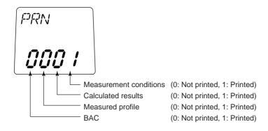
**NOTE** "0111" has been factory-set for the print items (the measurement conditions, calculated results, and measured profile are printed, and the BAC is not printed).
