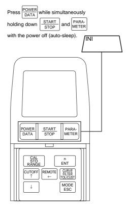
Moving to the detector position display mode (The SJ-201R requires another operation. For detailed information, refer to "3.4.5 Displaying the detector stylus position".)
