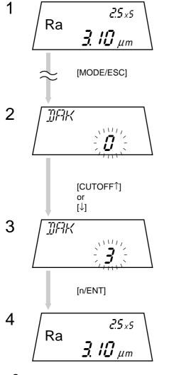
Press the [MODE/ESC] key several times in the measurement mode until "DAK" (measurement result output setting mode) is displayed.
