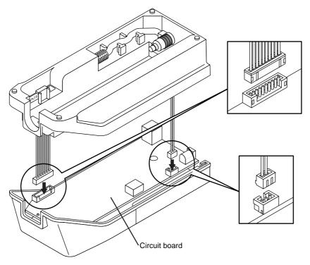
**IMPORTANT** Exercise care not to have the cable pinched by the PCBs or by the upper and lower sections of the display unit when fitting the lower section to the upper section. Cable or display unit breakage may result.
