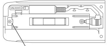
Drive/detector unit retaining plate
