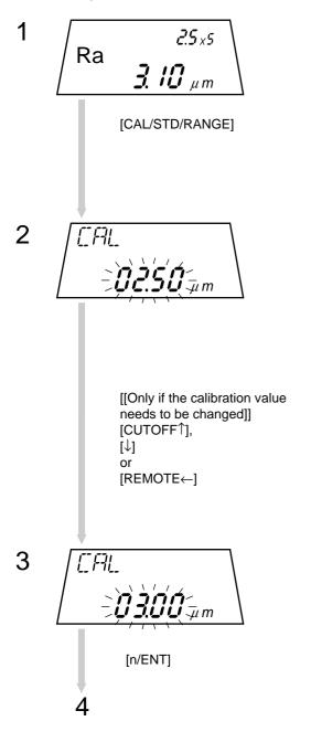
Press the [CAL/STD/RANGE] key in the measurement mode.
