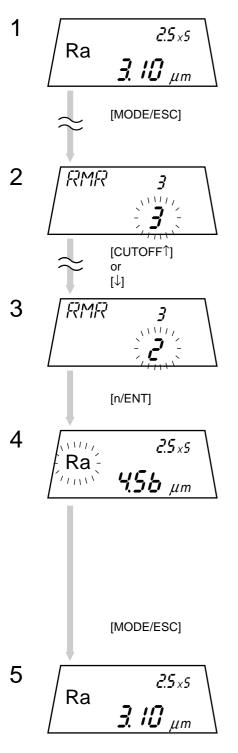
Press the [MODE/ESC] key several times in the measurement mode until "RMR" (saved data call and delete setting mode) is displayed.
