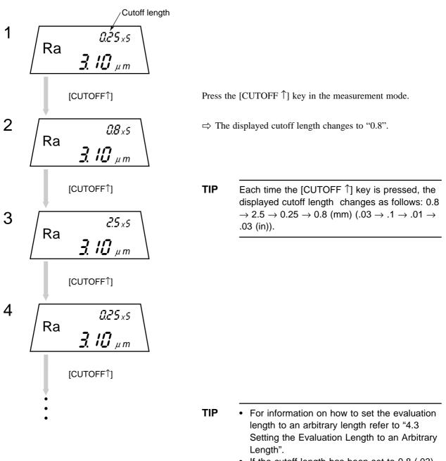
If the cutoff length has been set to 0.8 (.03), either 0.5 mm/s (.02in/s) or 0.25 mm/s (.01in/ s) can be selected as the traversing speed. See also "4.11 Modifying the Traversing Speed".
