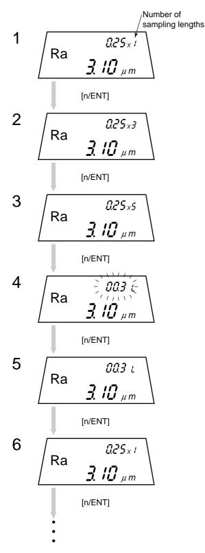
Press the [n/ENT] key in the measurement mode.
