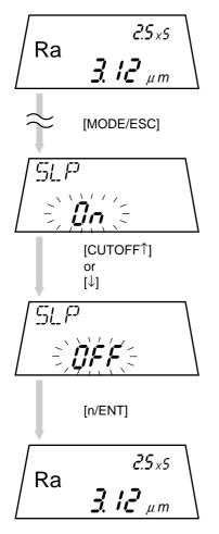
Press the [MODE/ESC] key a several times in the measurement mode.
