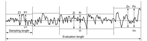
• Profile peak/highest peak and profile valley/deepest valley of assessed profiles A portion that projects upward (convex) from the mean line of the assessed profile is called the "profile peak", and that which projects downward (concave) is called the "profile valley".
