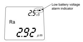
• If the battery power is supposed to be exhausted after having performed significant times of measurements although the low battery voltage alarm indicator is not flashing.
