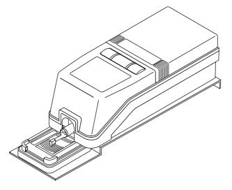
3. Set the SJ-201P so that the detector traversing direction is perpendicular to the cutter mark of the precision roughness specimen.
