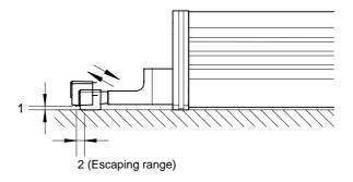
**NOTE** The SJ-201R cannot use the retraction function due to the front escape type.
