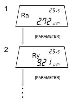
A measurement result (on parameter Ra) is being displayed now.
