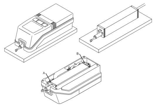
3. Confirm that the stylus is in proper contact with the measured surface. In addition, confirm that the detector is parallel to the measured surface.
