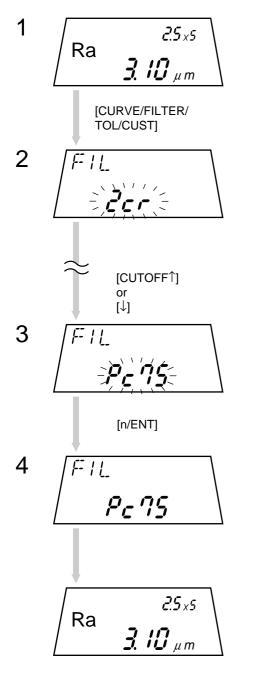
Press the [CURVE/FILTER/TOL/CUST] key several times in the measurement mode.
