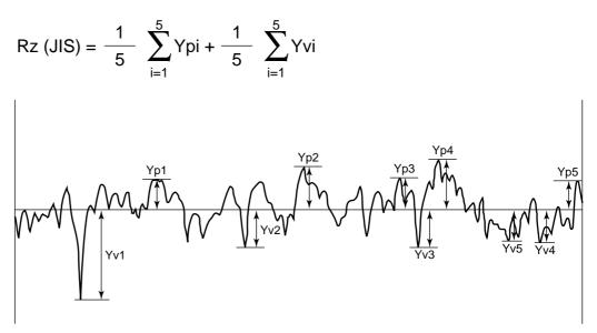
• Profile peak/highest peak and profile valley/deepest valley of assessed profiles A portion that projects upward (convex) from the mean line of the assessed profile is called the "profile peak", and that which projects downward (concave) is called the "profile valley".
