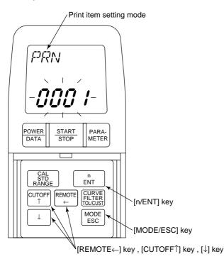
In the print item setting mode, the LCD shows a 4-digit number that indicates whether to print each of the four print items. The following shows the meaning of each digit number.
