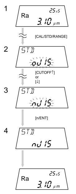
In the measurement mode press the [CAL/STD/RANGE] key twice.
