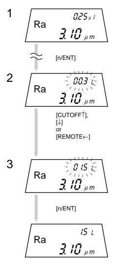
In the measurement mode press the [n/ENT] key until an "L" appears in place of the number of sampling lengths.
