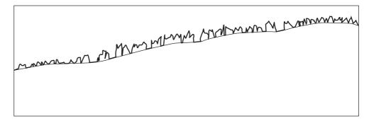
3. The second mean line is obtained with respect to the data obtained in the step 2.
