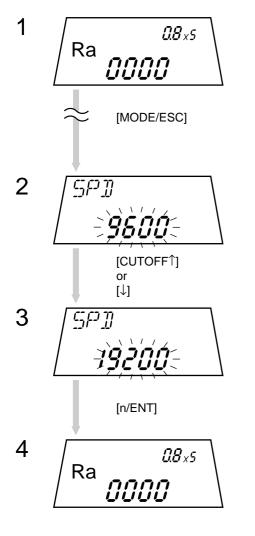
Press the [MODE/ESC] key several times in the measurement mode until "SPD" (RS-232C baud rate setting mode) is displayed.
