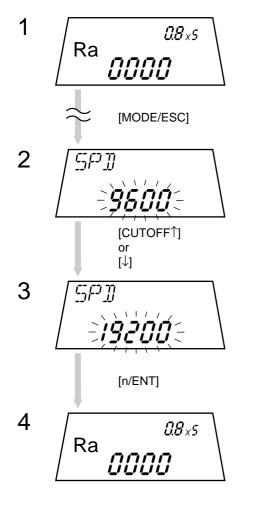
Press the [MODE/ESC] key several times in the measurement mode until "SPD" is displayed.
