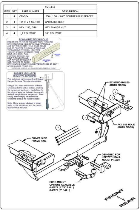
1) Support and lower the exhaust by removing (2) rubber isolators mounted to the muffler. Remove the panels from behind the rear wheels by removing (2) hex nuts using a 10mm socket and (2) screws with a 7/32" socket. Set panels aside for later installation.
