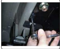
6) Raise the exhaust back into position and reinstall rubber isolators and exhaust bezels if removed.
