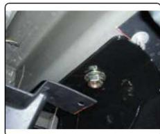
5) Torque all 1/2" fasteners to 110 lb-ft. Reinstall the trimmed underbody panels onto the vehicle using the hardware removed in step 1.
