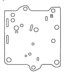
Install the end plate bolts loosely. LAST THING: Tighten plate bolts.
