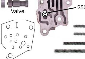
Install the end plate bolts loosely. LAST THING: Tighten plate bolts
