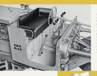
Caterpillar mechanical power controls give range and speed to blade movements not found in any other type of control. As well as increasing versatility, these controls help the operator get the job done more quickly and economically. Powered directly from the engine for positive action, Cat mechanical controls are simple in design and give dependable service without day-to-day maintenance.
