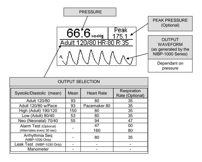
**PRESSURE GRAPH SCREEN** – This screen provides a graph of the pressure, as well as, the pressure, peak pressure and output selection
