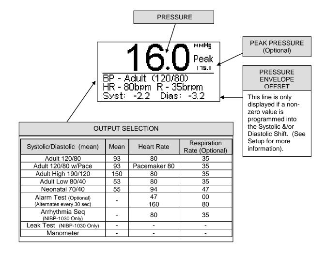
**OUTPUT WAVEFORM SCREEN** – This screen shows the pressure, peak pressure, output selection, and output waveform.
