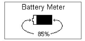
Batteries charge from provided AC power adapter. The charge time is about 4 hours from full discharge. While the batteries are charging, the display will flash "charging."
