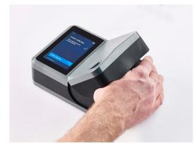
As of 2017, the original idea to non-invasively glucose monitor using Raman spectroscopy became highly within reach, since the technology had matured enough to lead to the design of the first prototype to be used in trials for market approval in Europe.
