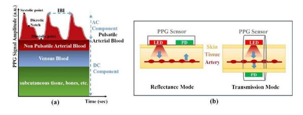
The principle of heart rate measurement used in "smart" bands differs from what is used in conventional medical devices with mechanical or electrical action. This is due to the sensors built into the inner side of the bracelet. The method of photoplethysmography is used for their work, which allows you to determine changes in blood volume using optical radiation. When contracting, the heart
