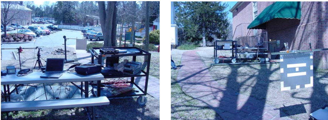
Figure A4: Luna experimental set-up moved from laboratory to outdoors to study the signal-to-noise ratio and effect of ambient noise that may interfere with weapons detection data in a real test situation.
