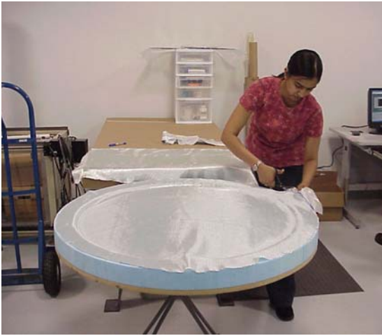
Figure 15: A picture of the elliptical receiver dish mold under fabrication is shown here.
