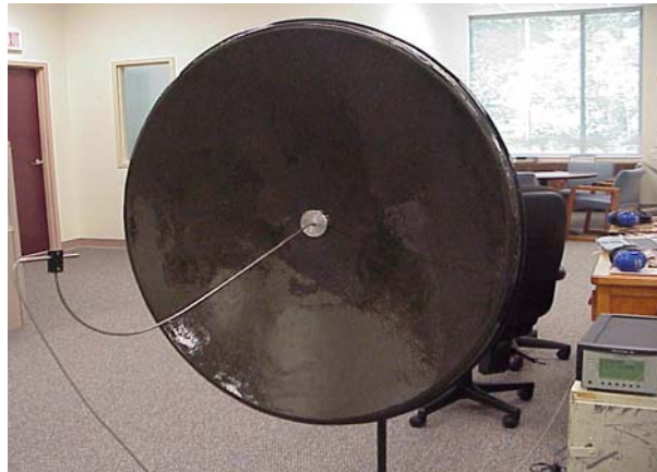
Figure 16: A picture of the elliptical receiver dish with a sensitive microphone at its focus.
