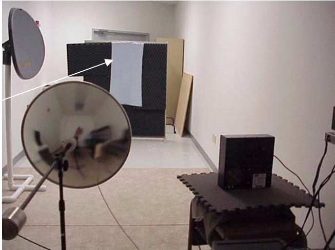
Figure 18: Experimental set-up for concealed weapons detection using the parabolic receiver dish and the Hypersonic Sound transmitter.
