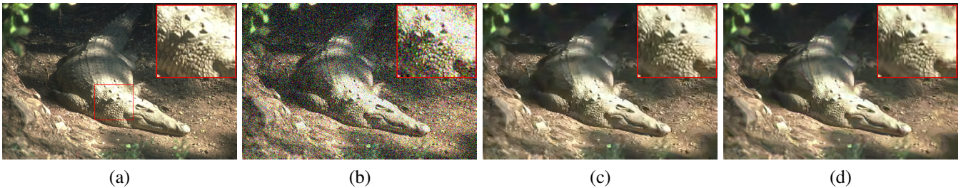
Figure 5. Color image denoising. (a) Original image, (b) Noisy image corrupted with Gaussian noise ( \sigma = 50 ); PSNR = 14.15 dB. (c) Denoised image using \text{CNLNet}_{5 \times 5}^3 ; PSNR = 26.06 dB. (d) Denoised image using CBM3D [7]; PSNR = 25.65 dB.
