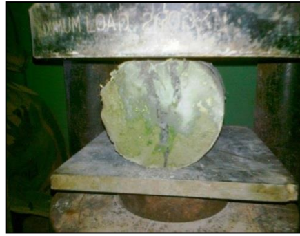
Fig. 3. Cylinder specimen under splitting tensile strength test.
