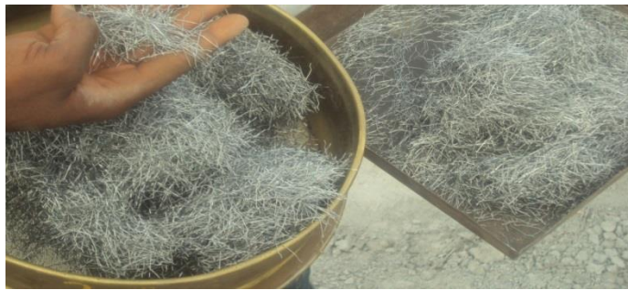
Fig. 1. Hooked-end type steel fibre used.
