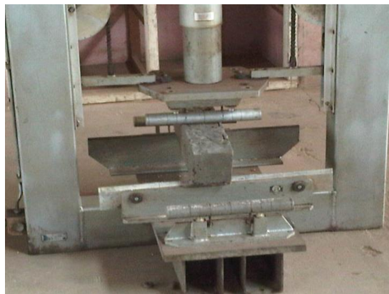
Fig. 2. Concrete beam under flexural strength test.
