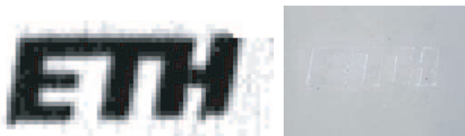
Figure 4.6: Phase resolved terahertz image of a transparent sample. The contrast is due to the different transit times of the terahertz pulse through one or two layers of overhead projector slides.
