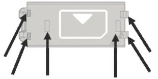
Insert the chip card into the lid according to the describing picture on the inside of the lid. Press until there is a clicking sound and the card sits tight in the lid.
