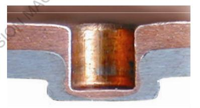
Clinching uses no heat, rivets, screws or adhesives
