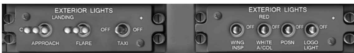
Figure 14.1.1. Exterior Light Control Panels
