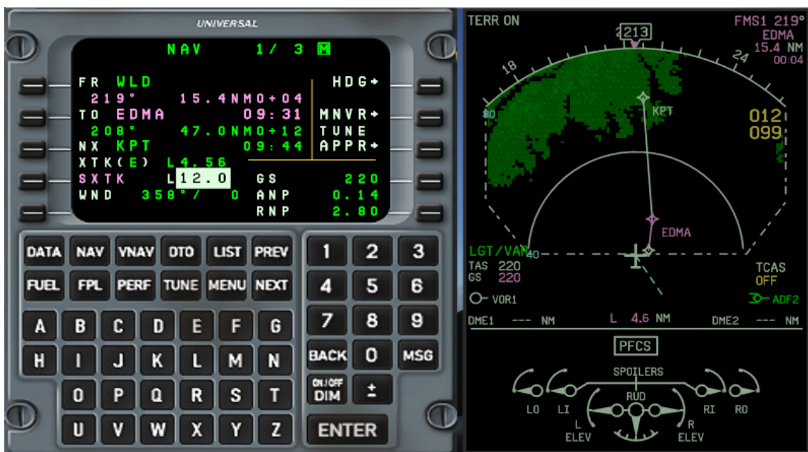
Figure 16.9.8.7. SXTK mode illustration
