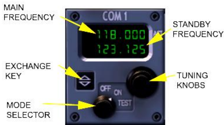
Figure 6.9.1. Standby COM Panel
