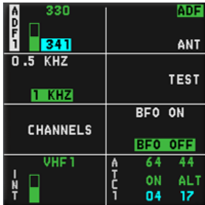
Figure 16.3.1. The ADF expanded page
