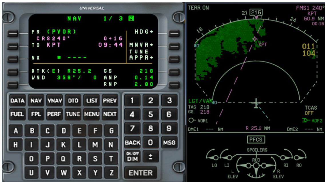
Figure 16.9.8.6. PVOR operation illustration
