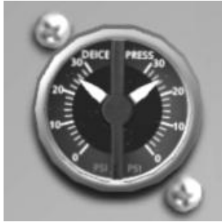
Figure 11.1.2. Deice Pressure Indicator
