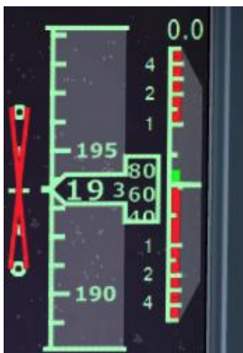
Figure 16.6.2.3. The Resolution Advisory indication on the PFD.
