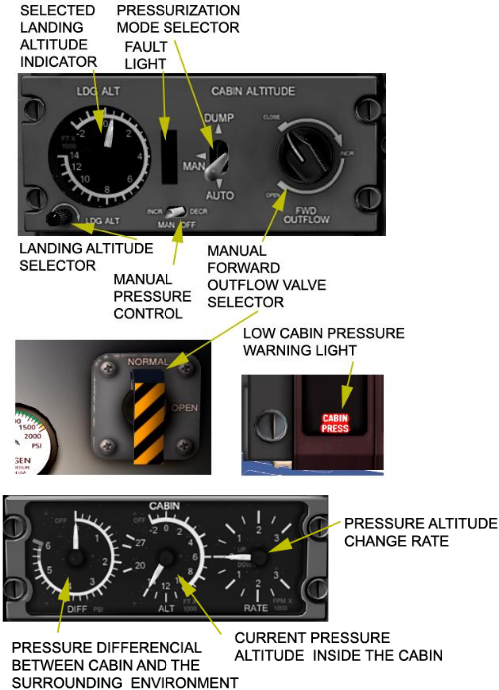
Figure 4.1.2. Pressure controls and indications
