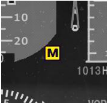
Figure 16.3.1. The Marker Indication
