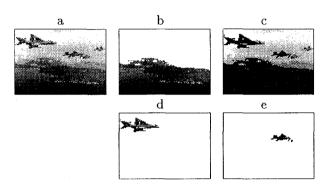
Figure 7: (a) shows a 77x107 color image. (b)-(e) show the components of the partition with Ncut value less than 0.04. Parameter settings:  $\sigma_I = 0.01$ ,  $\sigma_X = 4.0$ , r = 5.
