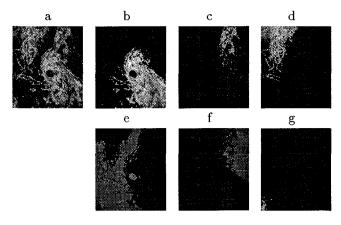
Figure 6: (a) shows a 126x106 weather radar image. (b)-(g) show the components of the partition with Ncut value less than 0.08. Parameter setting:  $\sigma_I = 0.005$ ,  $\sigma_x = 15.0$ , r = 10
