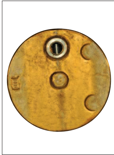
By Comparison – Flattened disc/boss areas of vertical disc design
