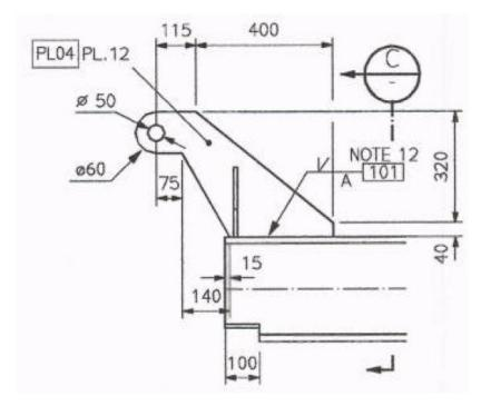
Figure H.1 – Typical installation arrangement for installation of hoists and trolley with self weight up to 500 kg. Special consideration of installation arrangement capacity shall be given to power driven hoists and beams with large SWL.
