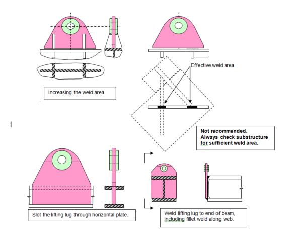
Figure J.3 - Welded connections
