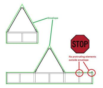
Figure F.1 - Envelope of unit represented by frame and sling arrangement
