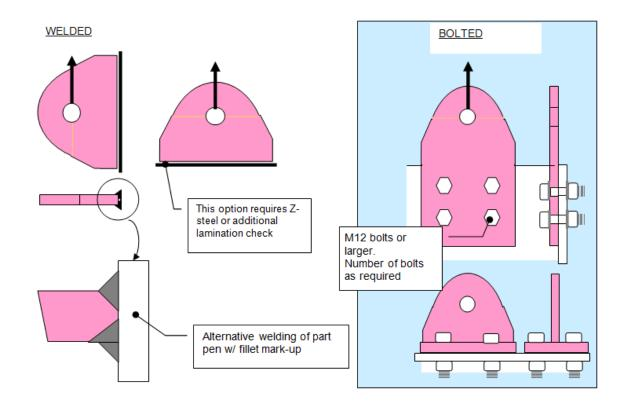
Figure J.2 - Welded/bolted connections
