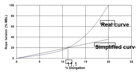
Figure I.1 – Rope static stiffness curve
