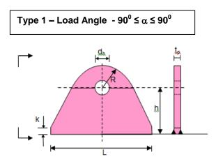
Dimensions in mm  $d_h = 1,03 \cdot d) + 2$  (Minimum hole diameter)  $1,3 \cdot d_h < R < 1,8 \cdot d_h$   $0,75 \cdot w_s \le t_p \le 0,9 \cdot (w_s - 3)$   $2.2 \cdot d_h \le h \le 2.4 \cdot d_h$   $2.4 \cdot h \le L \le 2.7 \cdot h$  d = shackle bolt diameter  $w_s =$  inside width of shackle at bolt section  $\alpha =$  load angle relative to vertical Maximum hole diameter shall not exceed  $d_h+5\%$
