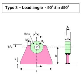
Figure J.7 - Lifting lug Type 3 geometry – Boss welded partly to plate
