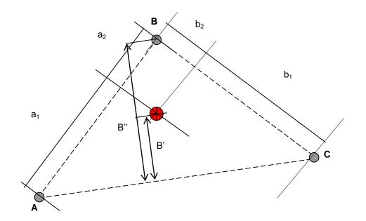
Figure F.5 - 3-point lift - Vertical design reaction PLP
