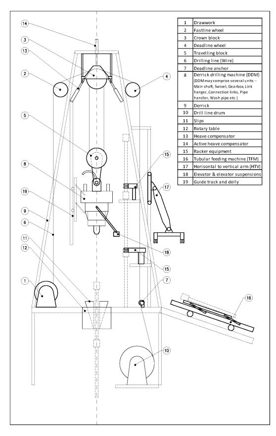
Figure D.1 – Conventional drawwork including top drive/DDM
