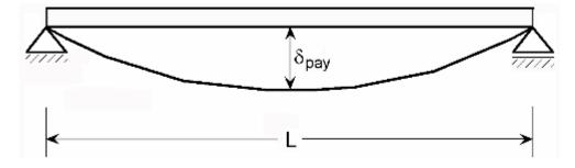
Vertical deformation,  $\delta_{pay}$ , of a runway beam relative to its supports (excluding load factors):
