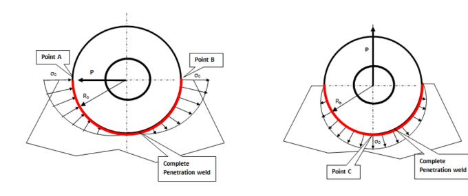
Figure J.11 – Horizontal loaded boss
