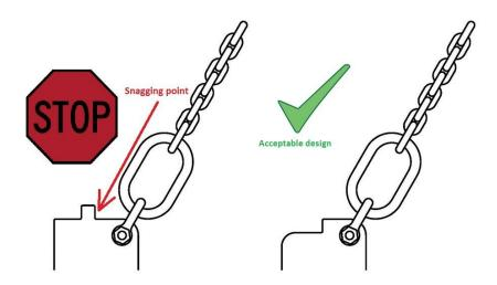
Figure F.2 – Example of unacceptable stacking pins representing a risk for entanglement to vessel, structure, sling set or other load
