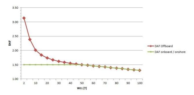
For all lifts from 50 tonnes to 100 tonnes designed according to this NORSOK standard, the dynamic facor DAF shall be selected with a linear reduction from 1,5 at 50 tonnes to 1,3 at 100 tonnes.
