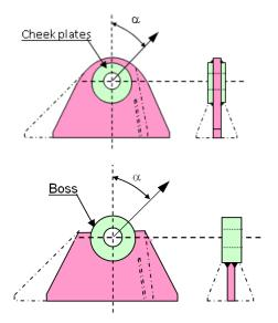
TYPE 2 (WLL < 55T)</th>Typical for shackles with WLL  $\leq$  55 TonnesLoad angle between  $-90^{0} \leq \alpha \leq 90^{0}$
