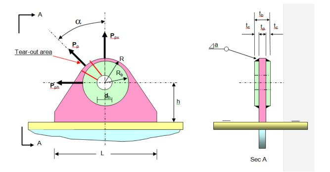
Figure J.8 - Design load components
