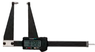
3M430A Electronic Digital Rotor Gauge • Range: 0-5.50" or 0-140mm • Graduations: .0005" or .01mm • Graduations: .001" • Includes storage case • Easy to read digital display with inch/metric conversion • Measures brake rotors and ball joints
