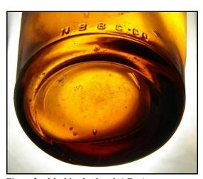
Figure 3 – Machine heelmark (eBay)
