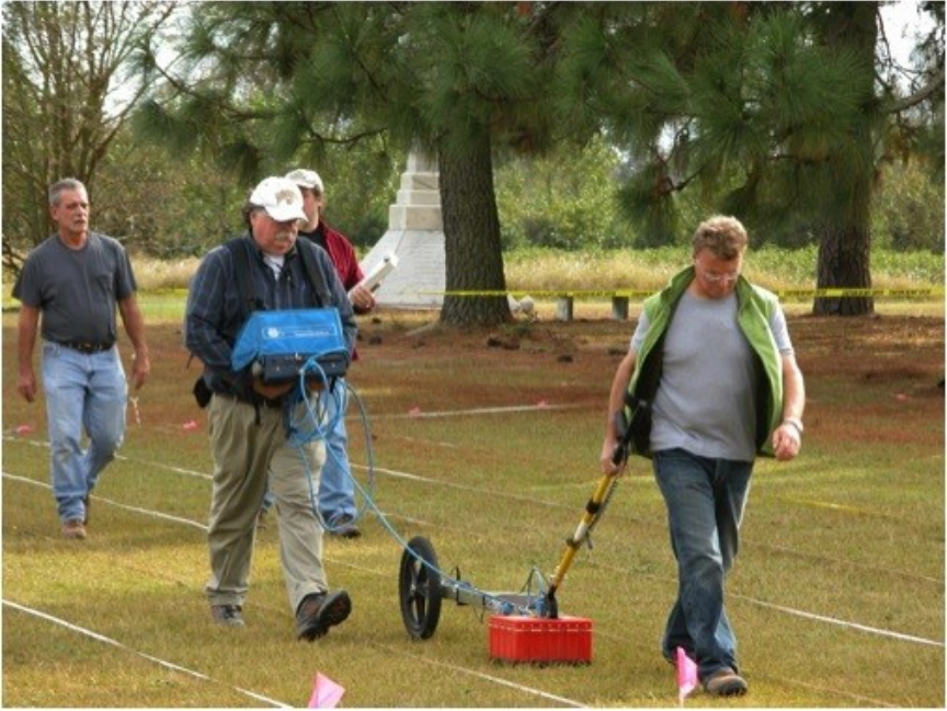
Figure 6. Collection of data in Study Area 1 using ground penetrating radar. Steve Thomas, host of The History Channel's Save Our History program, is pulling the radar sled while Ken Robinson reads the real time data output on his laptop. Also shown are Michael Murrow and Tom Beaman. View is to the southwest, with the commemoration monument visible in the background.
