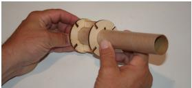
$\Box$  Locate the forward centering ring (the one with the two holes in it) and slide it onto the motor tube to one of the ½" marks. Using epoxy, bond the ring in place.
