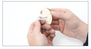
$\ \square$  Epoxy the bulkhead plate into the aft end of the coupler. Epoxy the coupler into the payload tube.
