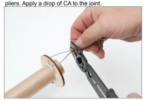
☐ Place the other loop/sleeve connector on the free end of the cable. Slide both of the heat shrink sections onto the cable. Make a 1-2" diameter loop and thread the free end back
