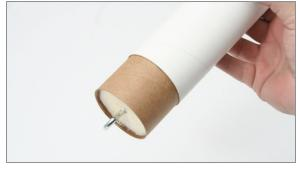
☐ Using a pencil and a straight edge, extend a 2" line on the payload tube. Locate one of the launch lugs and epoxy it in place. Fillet the lug for added strength.
