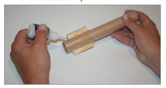
☐ Locate the one of the aft/mid centering ring (one with the four slots in it) and slide it onto the motor tube to mate with the key. Using epoxy, bond the ring in place. Repeat with the other ring in the mid location.
