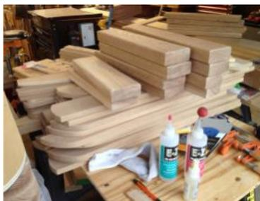
Okay, so now I had enough lumber. Onto some cutting. I made a cut list after analyzing all the templates. Most of the pieces were cut on the bandsaw about an 1/8" oversize. When I had everything cut, I mounted a flush trim bit in my router table and used double-stick tape to fasten the templates to the oak pieces. You have to be careful with your initial approach to the router bit. I had a few catches (yes,
