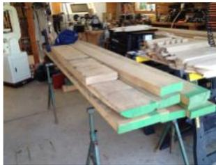
As I started laying out the templates on the white oak, I soon realized that most of the pieces needed to be cut from 1 1/2" thick stock. I ended up at Doll Lumber, where Eric Doll fixed me up with over 100 board feet of 8/4 white oak that was rough sawn. I took it home and spent an afternoon running it all through my planer. It took about 24 passes per board to get it down to 1 1/2". An added benefit was I ended up with over four heaping lawn cart loads of sawdust.
