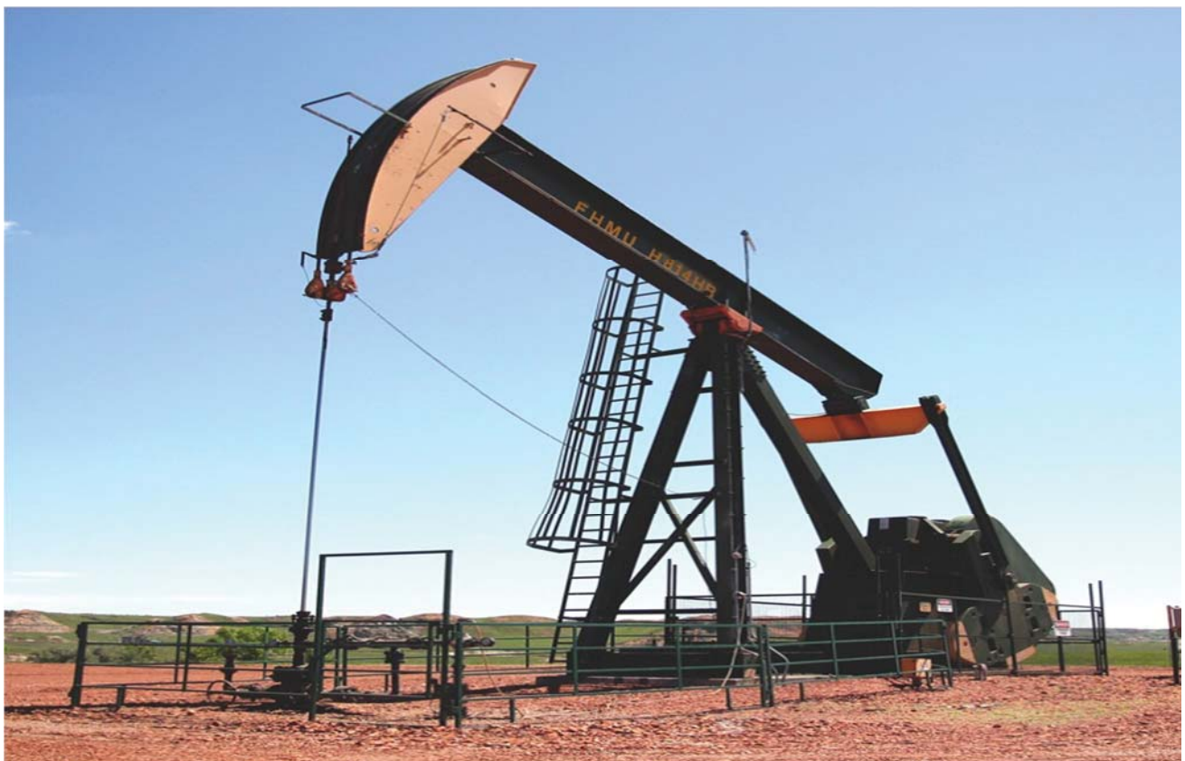
Oil pump jack, rural Billings County, North Dakota, Photo by Brian Austin (SHSND)
