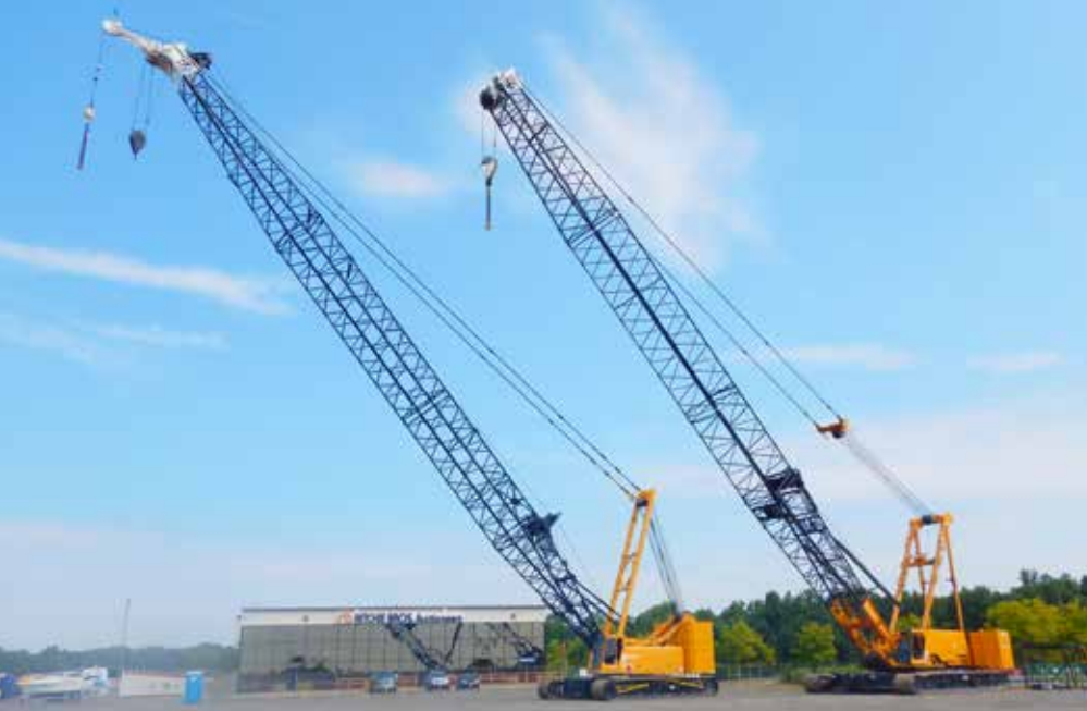
Manitowoc 2250 Series 3 300 Ton Self-Erecting & Manitowoc 999 275 Ton
